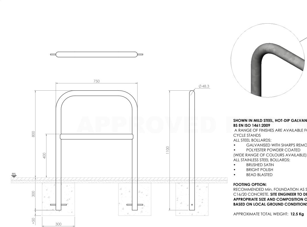
ROOT FIXED SHEFFIELD-TYPE CYCLE STAND HOT-DIP GALVANISED TO BS EN ISO 1461:2009 AS STANDARD CAN BE POLYESTER POWDER-COATED IN A RANGE OF RAL COLOURS - MID-RAIL SHOWN IN MILD STEEL, HOT-DIP GALVANISED TO A RANGE OF FINISHES ARE AVAILABLE FOR ALL - PINS FOR ROOT FIXING GALVANISED WITH SHARPS REMOVED
